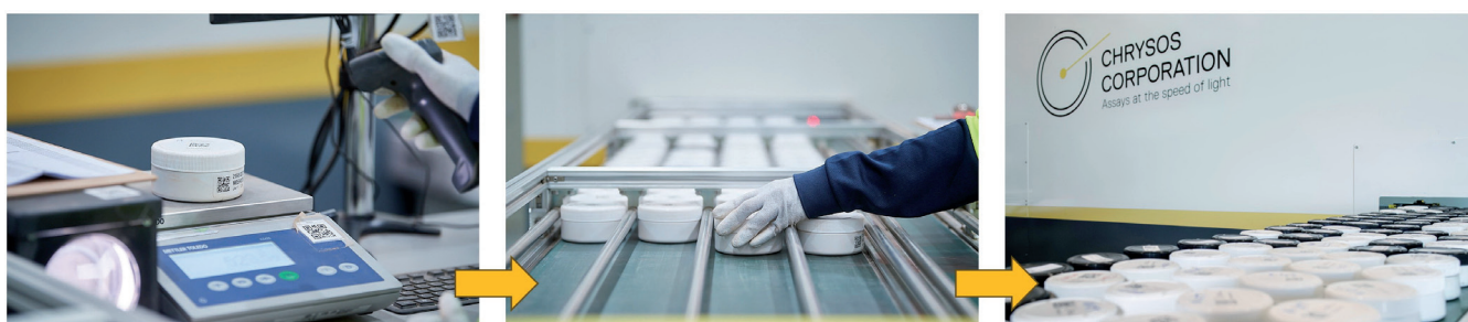
Fig. 3: Illustration of PhotonAssay™ process from left to right: sample jar registration and jar fill scanning; automatic feed of sample jars into the unit; and automatic outflow of jars from the unit.
